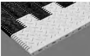
SERIES 400 NON SKID • Center-driven • Closed hinge • 2.00 in. (50.8 mm) pitch
