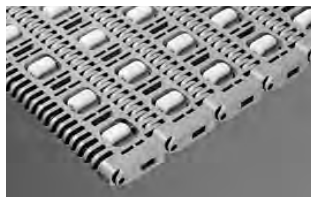
SERIES 400 TRANSVERSE ROLLER TOP • Center-driven • Closed hinge • 2.00 in. (50.8 mm) pitch
