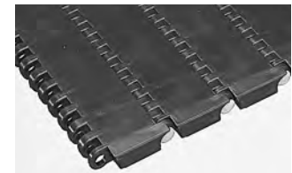
SERIES 900 • Center-driven • Closed hinge • 1.07 in. (27.2 mm) pitch
