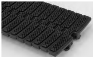
SERIES 4092 SQUARE FRICTION TOP • Hinge driven • Closed hinge • 1.00 in. (25.4 mm) pitch • Available width: 7.5 in. (191 mm)
