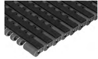
SERIES 1000 • Center/Hinge-driven • Closed hinge • 0.60 in. (15.2 mm) pitch
