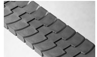
SERIES 4014 FLAT TOP • Hinge driven • Closed hinge • Sideflexing • 1.00 in. (25.4 mm) pitch • Available width: 83.8 mm (for parallel running at 85 mm)
