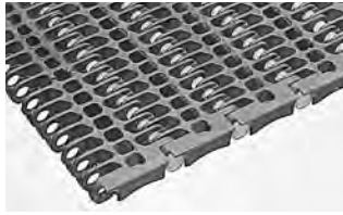
SERIES 100 • Center-driven • Open hinge • 1.00 in. (25.4 mm) pitch
