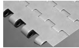
SERIES 1400 FLAT TOP • Center/hinge driven • Closed hinge • 1.00 in. (25.4 mm) pitch • Available widths: 6.0 in. (152 mm) and 9.3 in. (236 mm)
