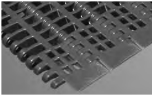
SERIES 900 FLUSH GRID • Center-driven • Open hinge • 1.07 in. (27.2 mm) pitch • Available widths: 4.7 in. (119 mm) and 6.0 in. (152 mm)
