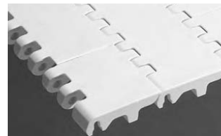
SERIES 1800 • Center-driven • Open hinge • 2.50 in. (63.5 mm) pitch
