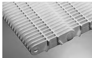
SERIES 400 • Center-driven • Open hinge • 2.00 in. (50.8 mm) pitch • Non flush edge
