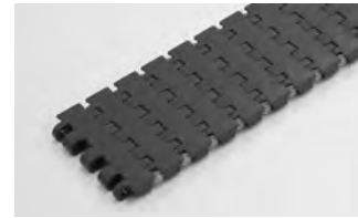
SERIES 1000 FLAT TOP • Center/Hinge driven • Closed hinge • 0.60 in. (15.2 mm) pitch • Available widths: 1.1 in. (29 mm), 1.5 in. (37 mm), 1.8 in. (46 mm), and 2.2 in. (55 mm)
