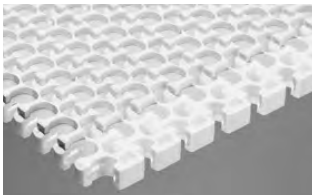
SERIES 2200 • Hinge-driven • Open hinge • Sideflexing • 1.50 in. (38.1 mm) pitch
