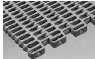
SERIES 2700 (2.2) • Hinge-driven • Open hinge • Sideflexing • 2.00 in. (50.8 mm) pitch
