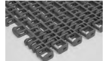
SERIES 2800 (1.6) • Hinge-driven • Open hinge • Sideflexing • 1.50 in. (38.1 mm) pitch
