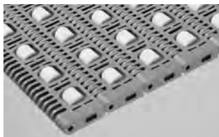
SERIES 400 ROLLER TOP • Center-driven • Closed hinge • 2.00 in. (50.8 mm) pitch
