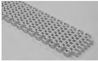
SERIES 2400 (2.2) • Hinge driven • Open hinge • Sideflexing • 1.00 in. (25.4 mm) pitch • Available width: 4.00 in. (101.6 mm)
