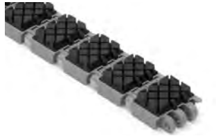
SERIES 900 SQUARE FRICTION TOP • Center driven • Closed hinge • 1.07 in. (27.2 mm) pitch • Available width: 1.1 in. (29 mm)
