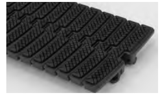
SERIES 4092 SQUARE FRICTION TOP • Hinge driven • Closed hinge • 1.00 in. (25.4 mm) pitch • Available width: 7.5 in. (191 mm)
