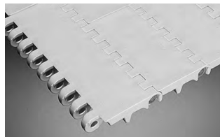
SERIES 800 • Center-driven • Open hinge • 2.00 in. (50.8 mm) pitch
