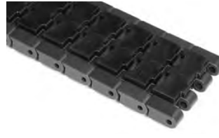
SERIES 1400 3.25" FLAT FRICTION WITH TABS • Center/hinge driven • Closed hinge • 1.00 in. (25.4 mm) pitch • Available width: 6.0 in. (152 mm)
