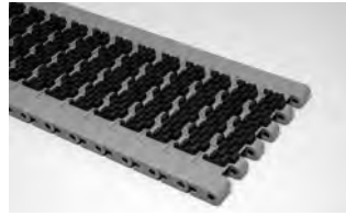
SERIES 1400 OVAL FRICTION TOP • Center/hinge driven • Closed hinge • 1.00 in. (25.4 mm) pitch • Available width: 6.0 in. (152 mm)
