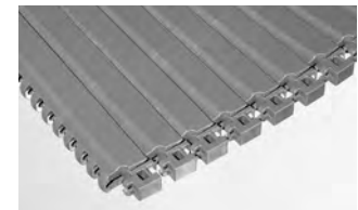
SERIES 2400 • Hinge-driven • Open hinge • Sideflexing • 1.00 in. (25.4 mm) pitch
