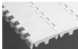
SERIES 1800 • Center-driven • Open hinge • 2.50 in. (63.5 mm) pitch • Flush edge
