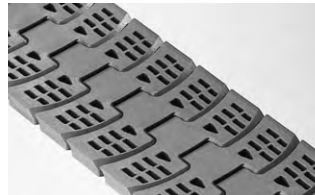
SERIES 4009 FLUSH GRID • Hinge driven • Closed hinge • Sideflexing • 1.00 in. (25.4 mm) pitch • Available width: 83.8 mm (for parallel running at 85 mm)
